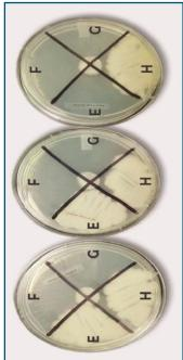
Extensive laboratory testing using various concentrations of MAPS<sup>®</sup> MATRIX47<sup>TM</sup> inoculated with Escherichia coli, Lactobacillus casei, Bacillus subtilis and Aspergillus niger prove that when MAPS<sup>®</sup> MATRIX47<sup>TM</sup> is used at the recommended rate, prevents the growth of bacteria and fungi within the surface coating.
